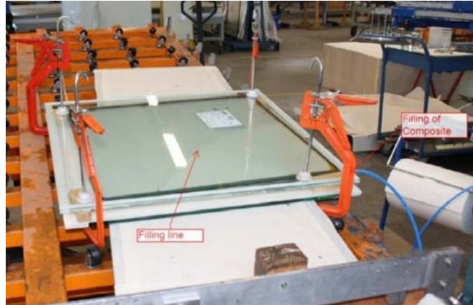
Fig. 7 GEWE Composite Lamination Process. Two lites of glass on being joined to create either an interior or exterior set of the IGU.
