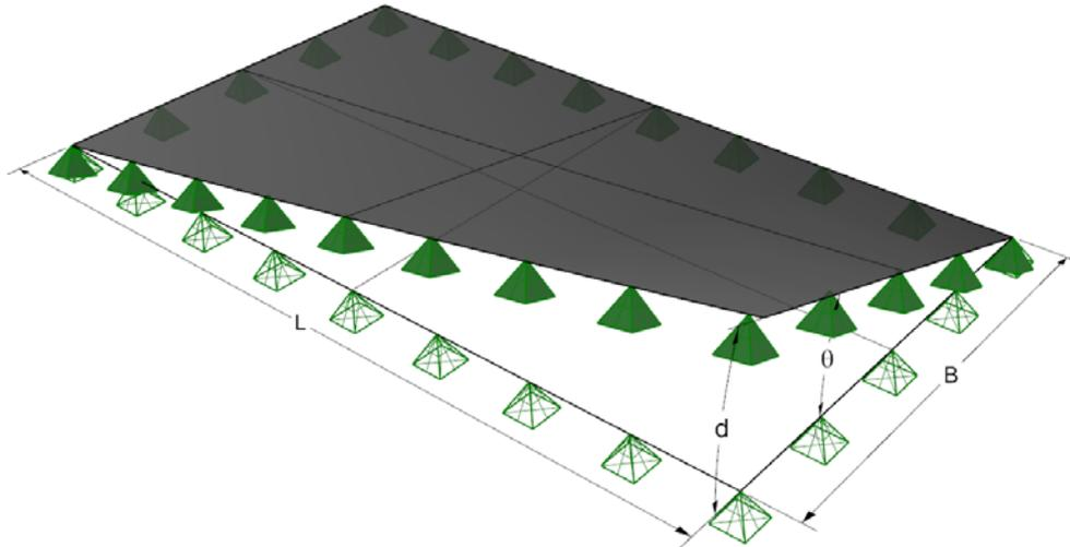
Fig. 3 Warping geometry nomenclature and support locations
