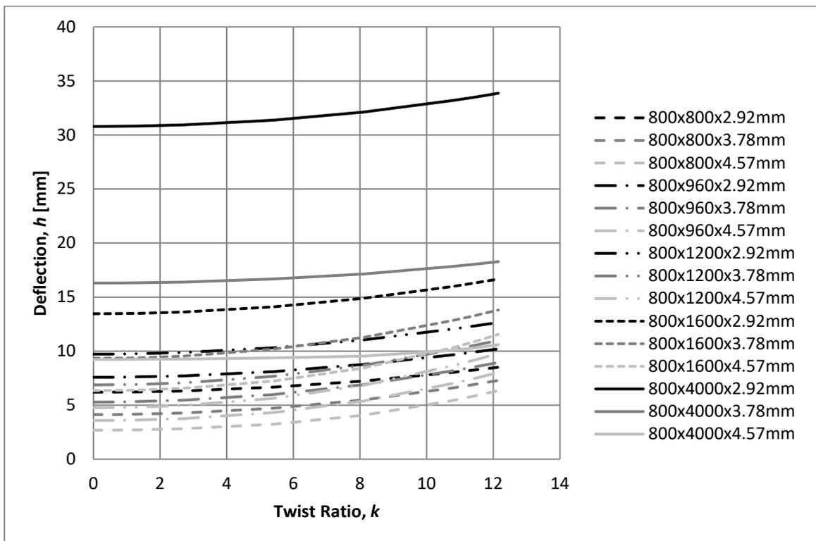
Fig. 7 Transverse deflection of 800mm wide specimens at 1.0 kPa
