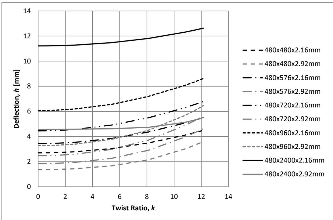
Fig. 5 Transverse deflection of 480mm wide specimens at 1.0 kPa
