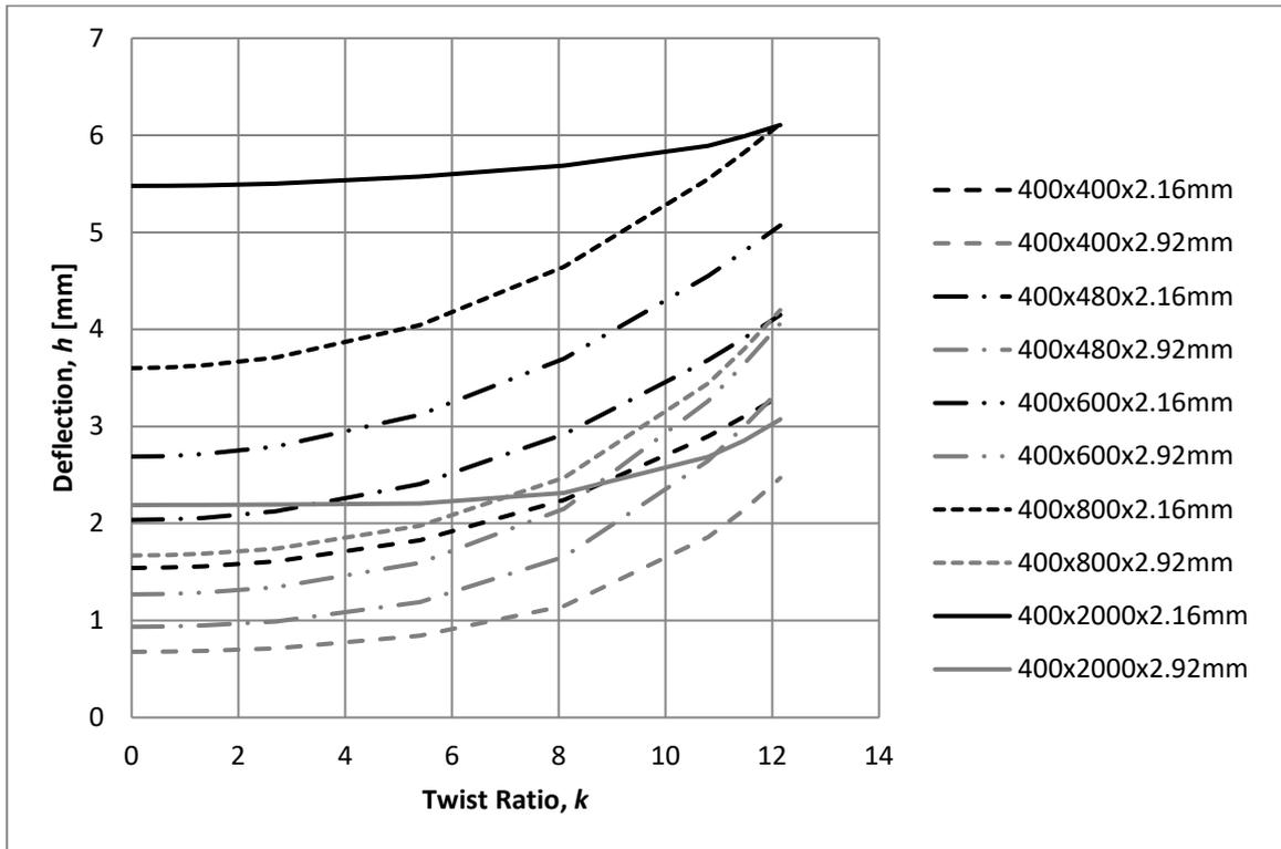
Fig. 4 Transverse deflection of 400mm wide specimens at 1.0 kPa
