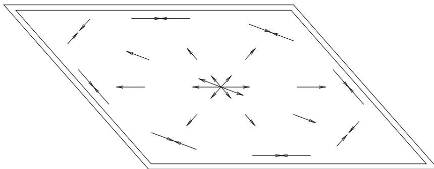
Fig. 2 Membrane tension resisted by membrane compression ring in thin plate
