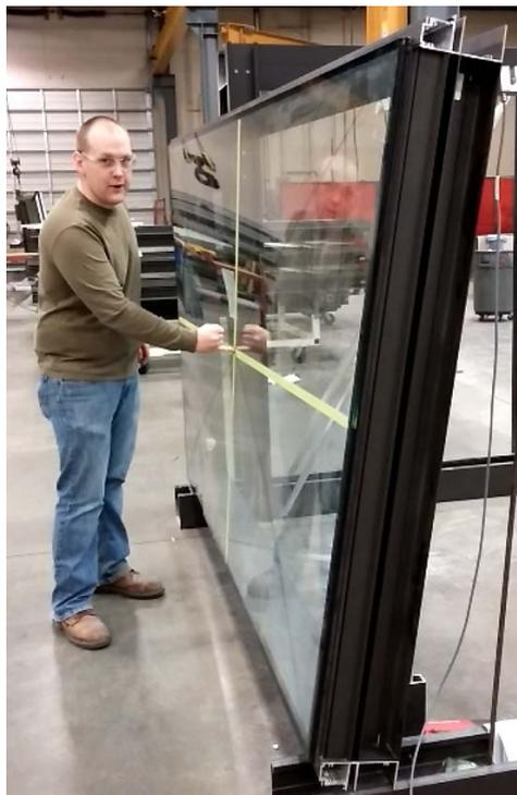
Fig. 9 Deformation of 9.02mm thick glass using the pinky finger method
