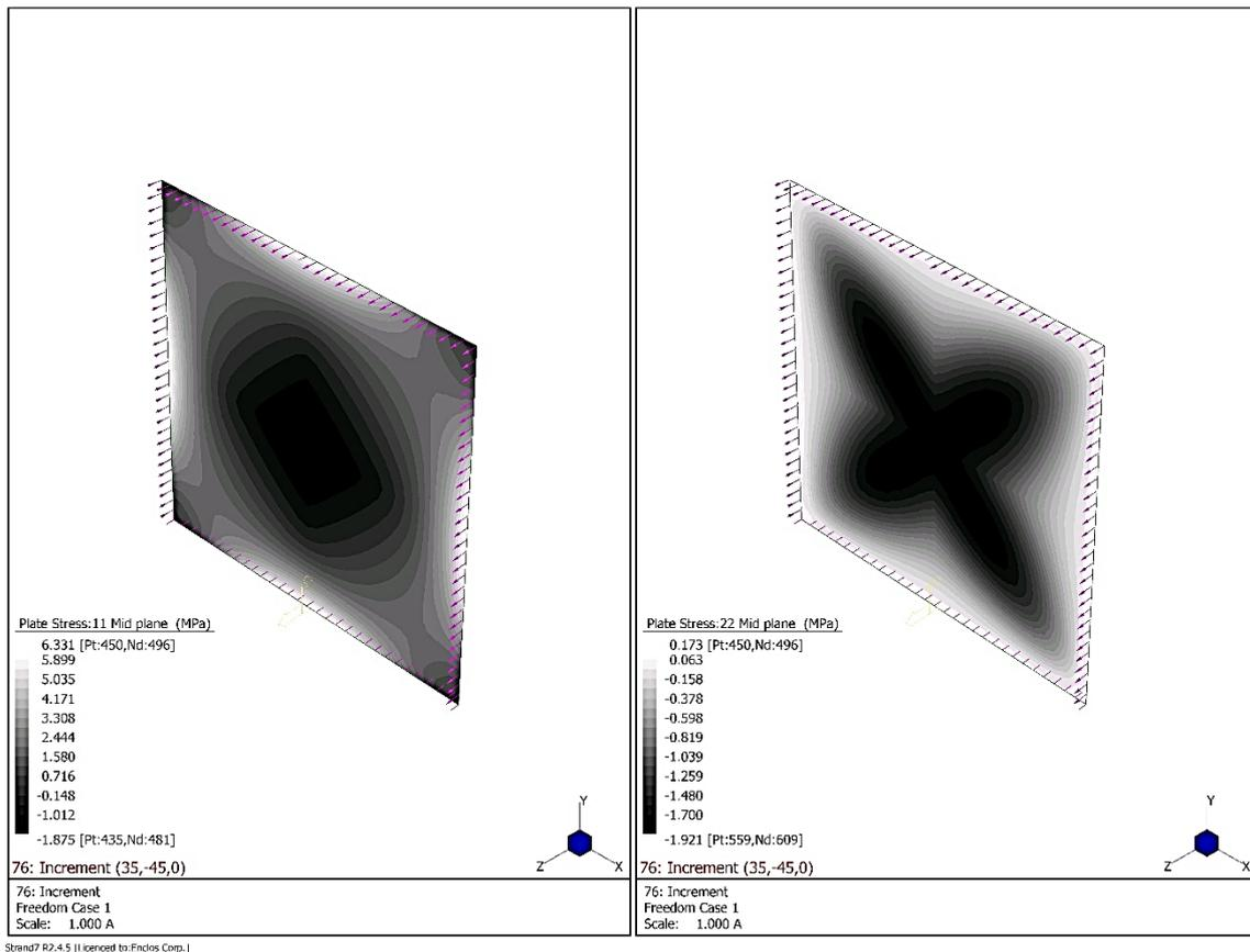
Fig. 10 Membrane stresses present in the  $1500\text{mm} \times 1500\text{mm}$  case including residual warping stress
