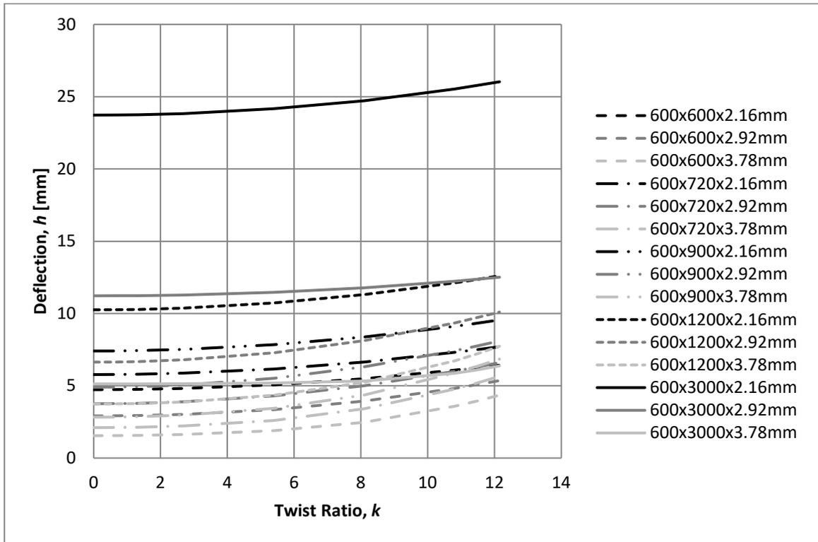
Fig. 6 Transverse deflection of 600mm wide specimens at 1.0 kPa
