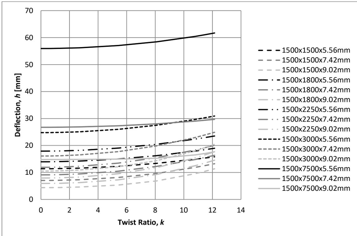
Fig. 8 Transverse deflection of 1500mm wide specimens at 1.0 kPa
