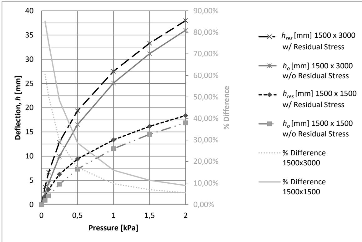
Fig. 11 Comparison of transverse deflection with and without inclusion of warping residual stresses
