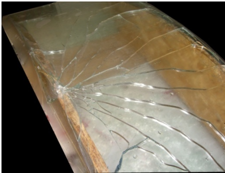
Figure 7a and b: Breakage pattern of curved heat strengthened glass panels (7a: not conform, 7b: conform to DIN EN 1863).
