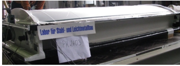
Figure 5: Vacuum test set-up.
