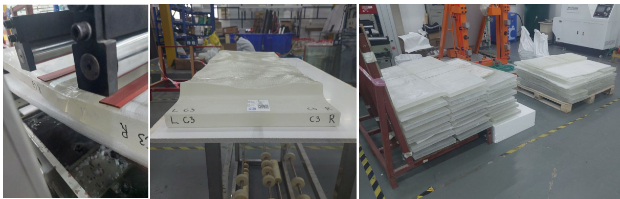
Fig. 4: Four-point bending test of undulated cast glass (82 valid tests in total)
