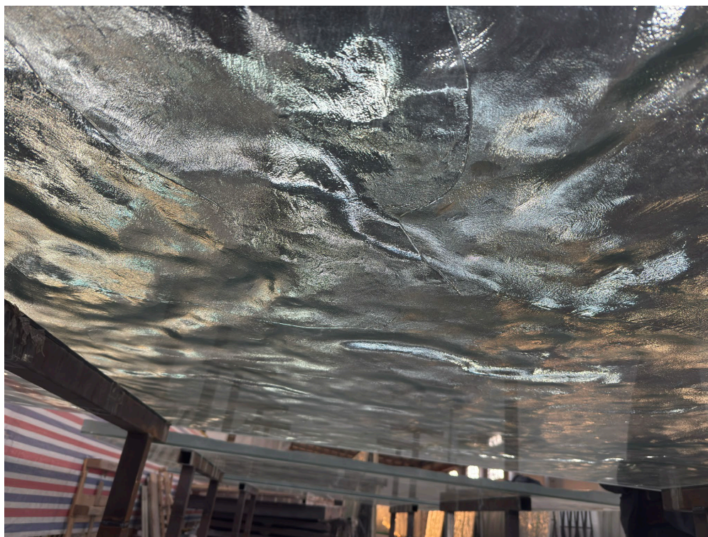
Fig. 1: Sample of borosilicate cast glass with average thickness of 70mm and size of 2.5m x 3.8m
