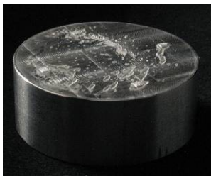
Figure 5: Delo glue, adhesive failure.
