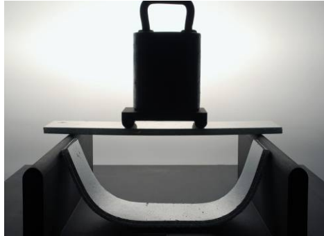
Figure 2: Laminated glass with and without embedded reinforcement in the damaged state.
