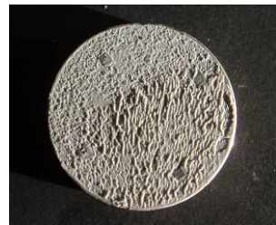
Figure 7: Sika glue, cohesive failure.
