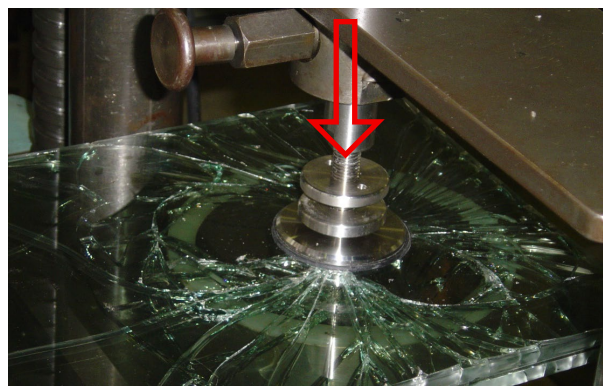
Fig. 5d: Lab sample testing, top ply always broke first.
