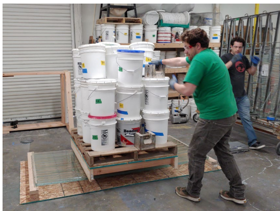
Fig. 7a: Informal 4-point bending validation test of full-scale art glass panel using copper slag weight in buckets (AN fused art glass | FT | AN fused art glass).
