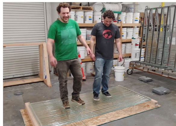
Fig. 7b: Residual capacity after initial fracture (Photos: Kerry Johnson Glass).
