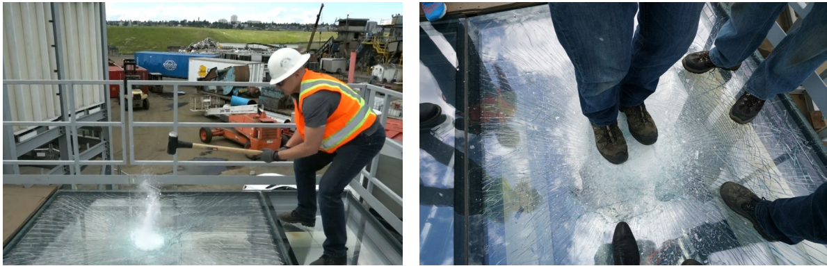
Fig. 6: Destructive testing of visual mockup.
