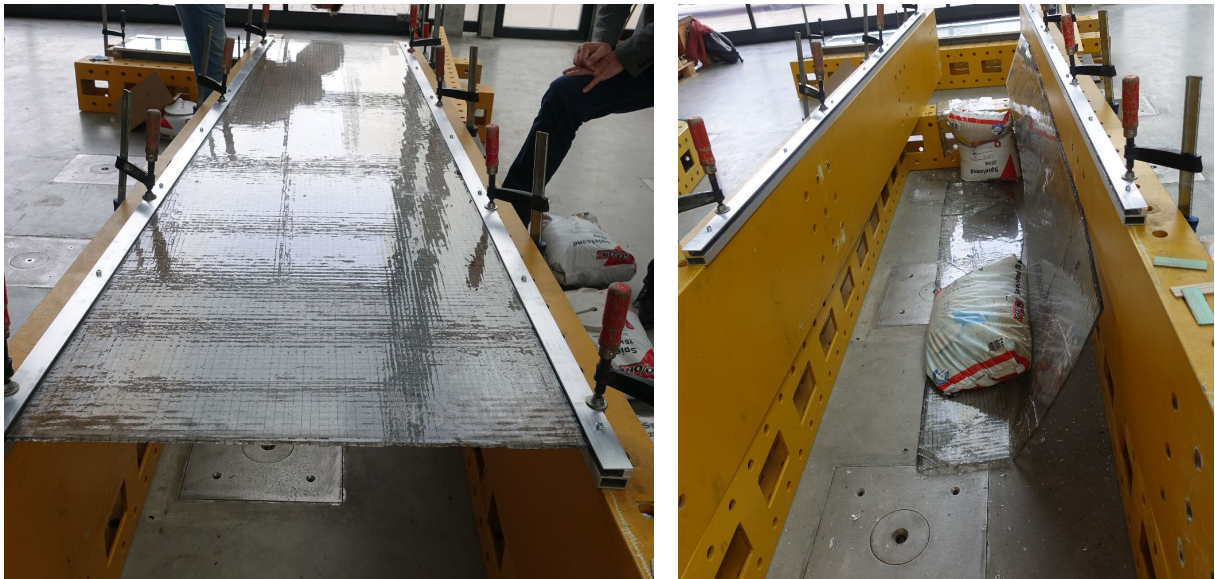
Fig. 10: Remaining load carrying capacity of wired glass, thickness 7mm.
