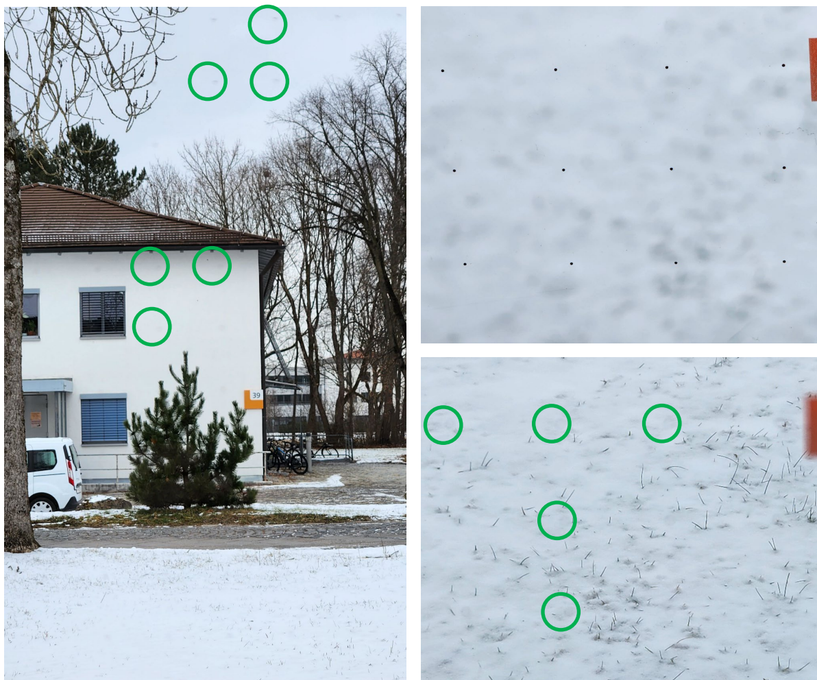
Fig. 6: Picture looking through VIG and detail view in two different focus distances, adhesive sticker (red) for reference. Marking (green circles) at locations of pillars inserted by hand on some spots only, selection random.
