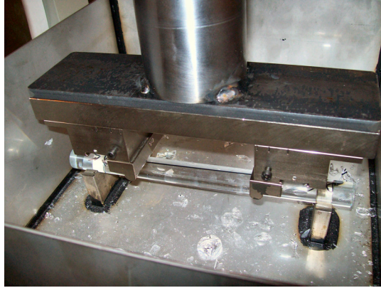
Figure 1: Test rig for glass bars.
