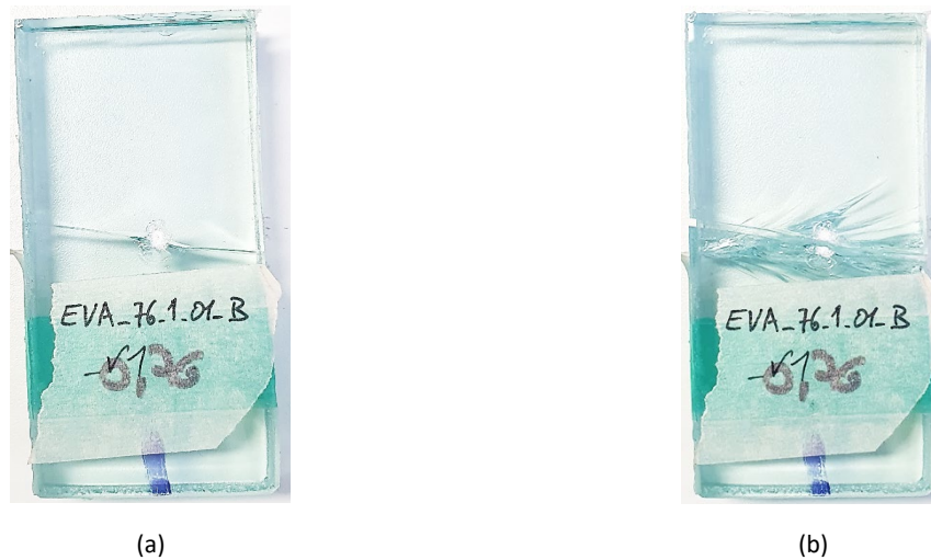
Fig. 6: Example of LG specimen: (a) with the preliminarily imposed crack and (b) after the cyclic protocol (bottom view).
