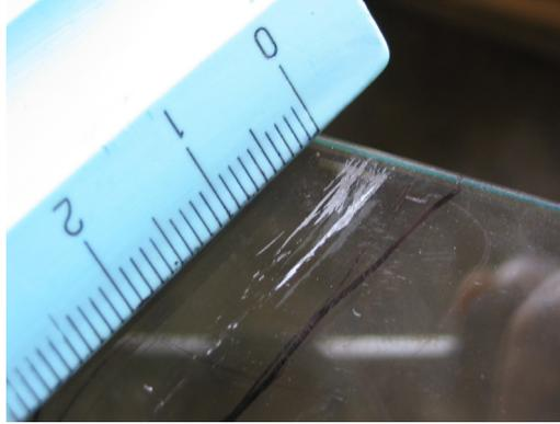
Figure 2: Some typical surface defects detected under the quality control of tempered glass plates in the production conditions.
