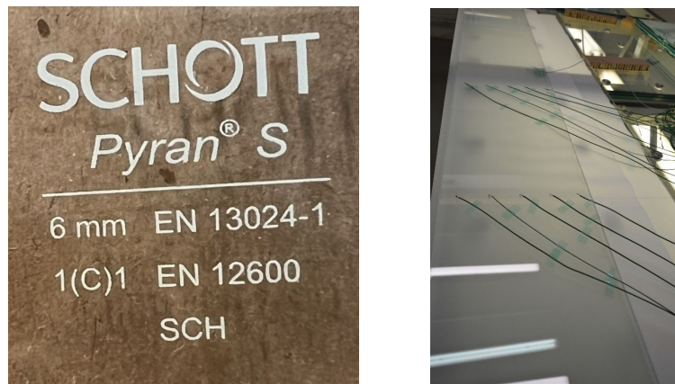
Fig. 3: Sample B: on the left, the PYRAN® S borosilicate glass label; on the right, the attachment of thermocouples and a measuring cable for recording deflection during the fire test.
