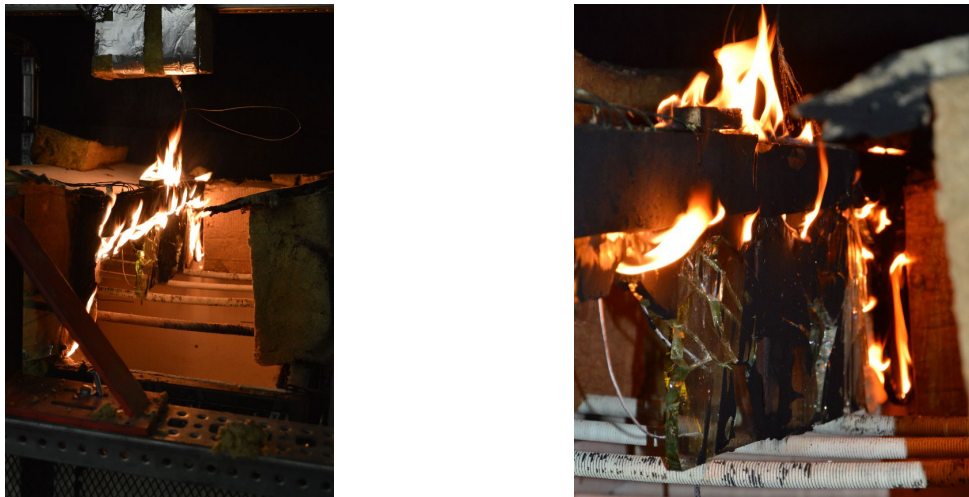
Fig. 9: Sample A – Deformation of the sample after the fire test.
