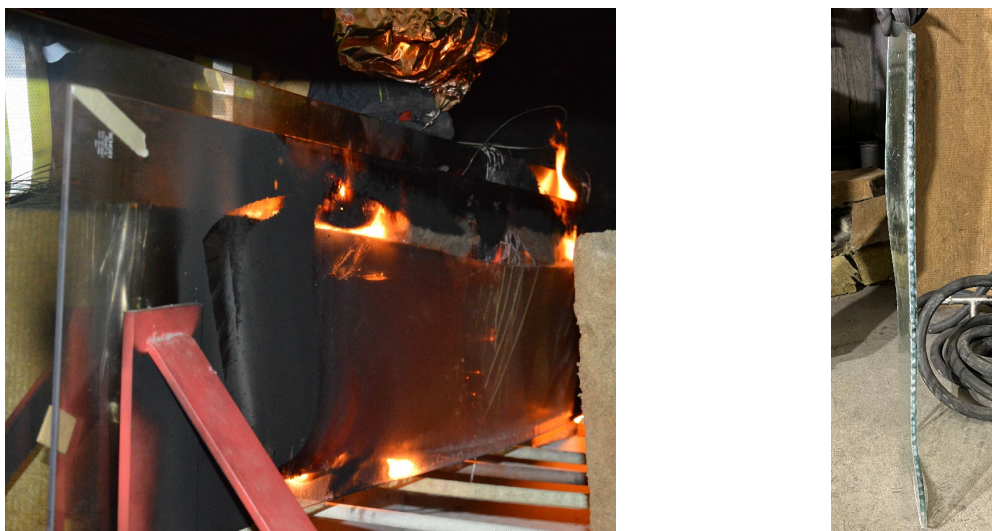
Fig. 10: Sample B – left: deformation of the sample after uncovering, right: deformation of the middle ply of float glass.
