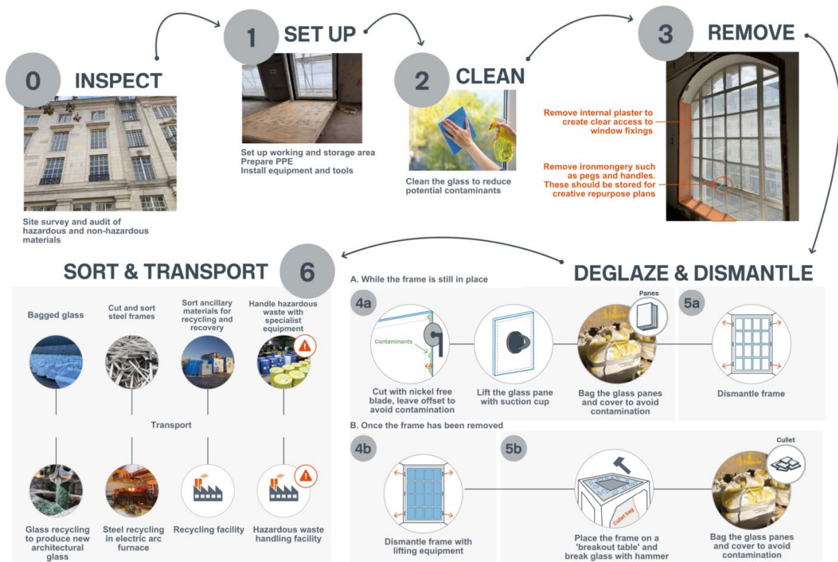
Fig. 5: Proposed dismantling process for windows being removed.
