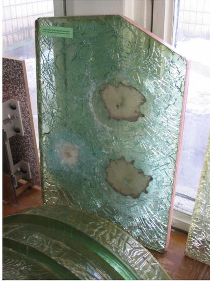
Figure 2. The multilayer bulletproof glass and composite rings made of sheet glass components.
