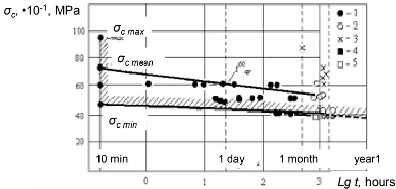
Figure 5. Durability curves for glass bars under contact axial compression.
