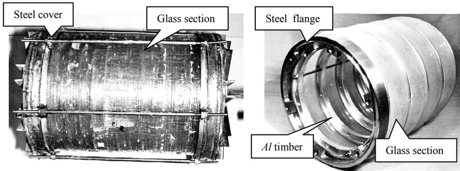
Figure 1. Strong composite glass shells intended for high external pressure.
