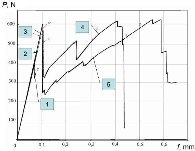
Figure 3. Deformation curves of the reinforced laminated glass composites under the bending. (The data were received together with Dr. Zemtsov M.P. and Dr. Skripchenko V.I.)
