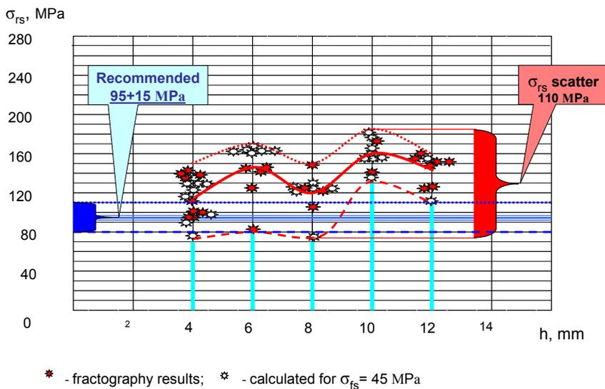
Figure 9 Residual compressive stress and quality of the hardened glass.
