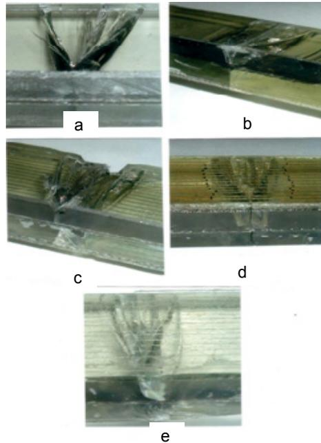
Figure 4. The character of specimen fracture of the reinforced triplex
