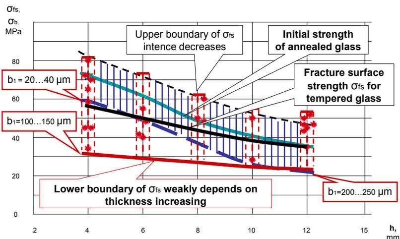
Figure 7 Influence of glass thickness on decreasing of glass surface mechanical resistance under the tempering conditions.
