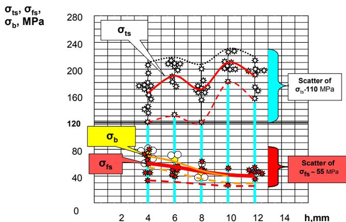
Figure 8. Fracture surface strength  $\sigma_{fs}$  and bending strength  $\sigma_b$  of tempered glass.
