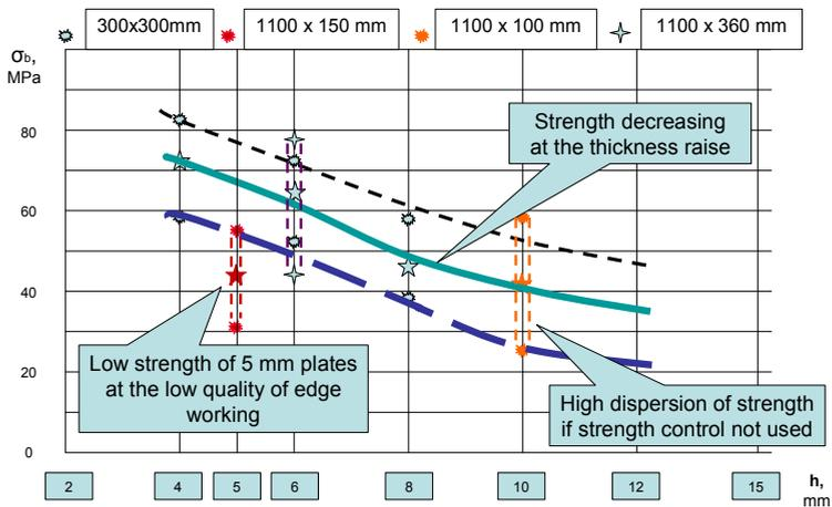
Figure 6. Quality and bending strength  $\sigma_b$  of annealed glass subject to thickness of the plates.
