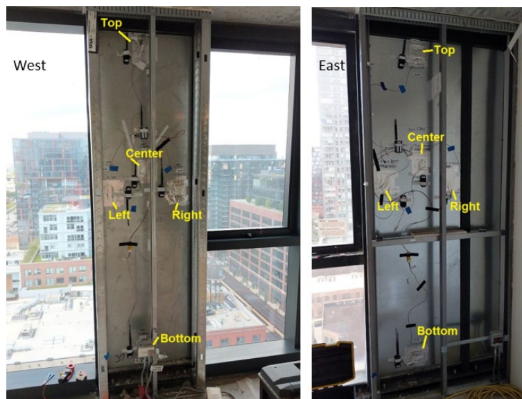
Fig. 6: Annotated photographs of instrumented spandrels in west- and east-facing units at the Chicago case study (photos by David Kosnik).
