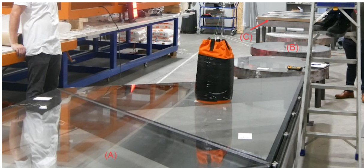
Fig. 4: Impact test on the rooflights. (A) Main rooflight. (B) Terrace rooflights. (C) Fire-rated rooflights.
