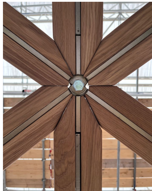
Fig. 7: Pre-assembly of the main roof at Bellapart's workshop.
