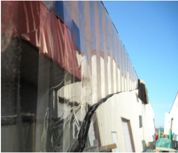
Fig. 3: Failed glass from site. Left: Thin layer of glass stuck to interlayer as evidenced by wavy reflection; Right: Fully detached flexible interlayer at one corner.
