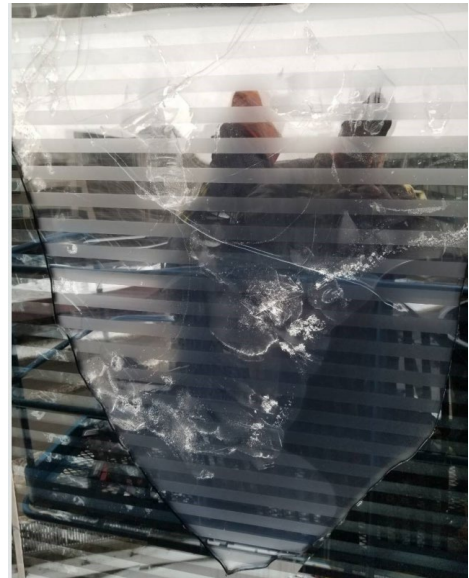
Fig. 4: Left: Salvaged site panel with fully detached interlayer and Ply 1 fragment suffering adhesive failure; Right: Failed site panel where a portion of the outer ply has detached from the interlayer, leaving a thin adhered layer of glass across a portion of the detached zone.
