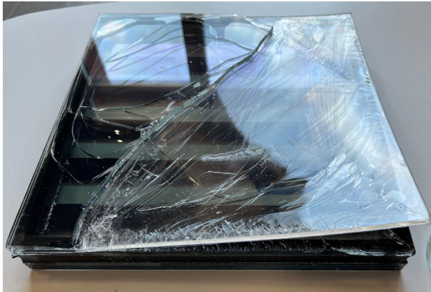
Fig. 9: Freezer tests compared with site glass. Left: freezer test thin layer of glass adhered to on surface (Mode II failure) and adhesive delamination bottom on #3 surface. Right, site sample
