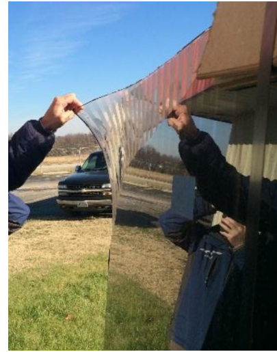
Fig. 3: Failed glass from site. Left: Thin layer of glass stuck to interlayer as evidenced by wavy reflection; Right: Fully detached flexible interlayer at one corner.
