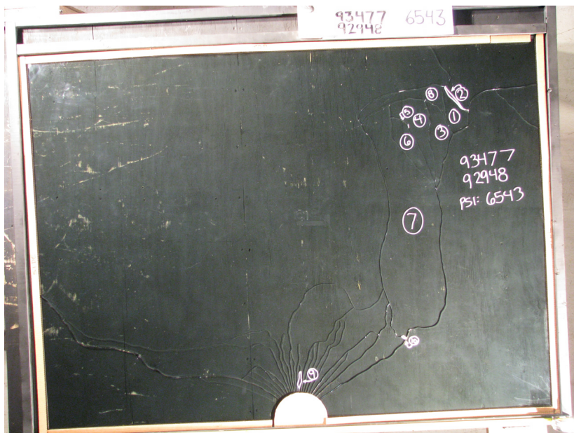
Figure 1: Example of tested lite with residual surface compressive stress of 45 MPa.
