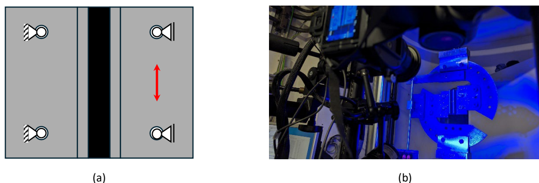
Fig. 2: (a) Static System of the Shear Tests; (b) Experimental Setup of the Cyclic Material Testing.
