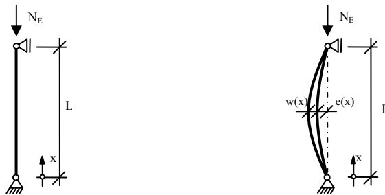
Figure 2: Origin, perfect and deformed imperfect system of a slim column, e(x) =imperfection, w(x) = bending ordinate.
