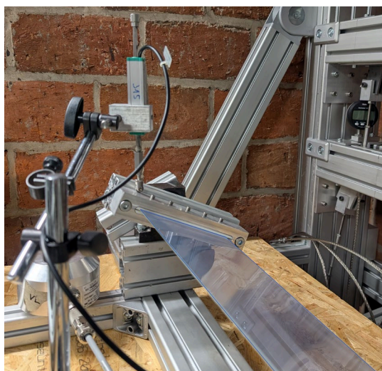
Fig. 4: Left: Specimen with displacement transducer after 850 hours of recovery. Right: Time-dependent recovery. Torsional angle over time.
