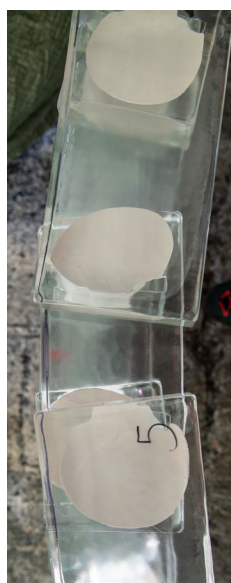
Fig. 13: The adhesive layer was deposited in the form of blobs, resulting in an interface of \approx 2 mm thickness.
