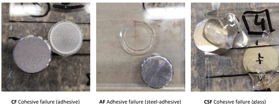
Fig. 17: Representative fracture surfaces of pull-off specimens: cohesive failure within the adhesive layer (CF), adhesive failure at the steel-adhesive interface (AF) and cohesive failure in the glass substrate (CSF) (from left to right).
