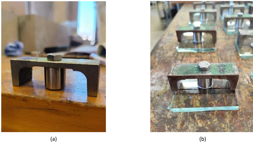
Fig. 2: Alignment bridge used during specimen preparation to ensure concentric dolly positioning and to control the nominal adhesive layer thickness (0.3 mm).
