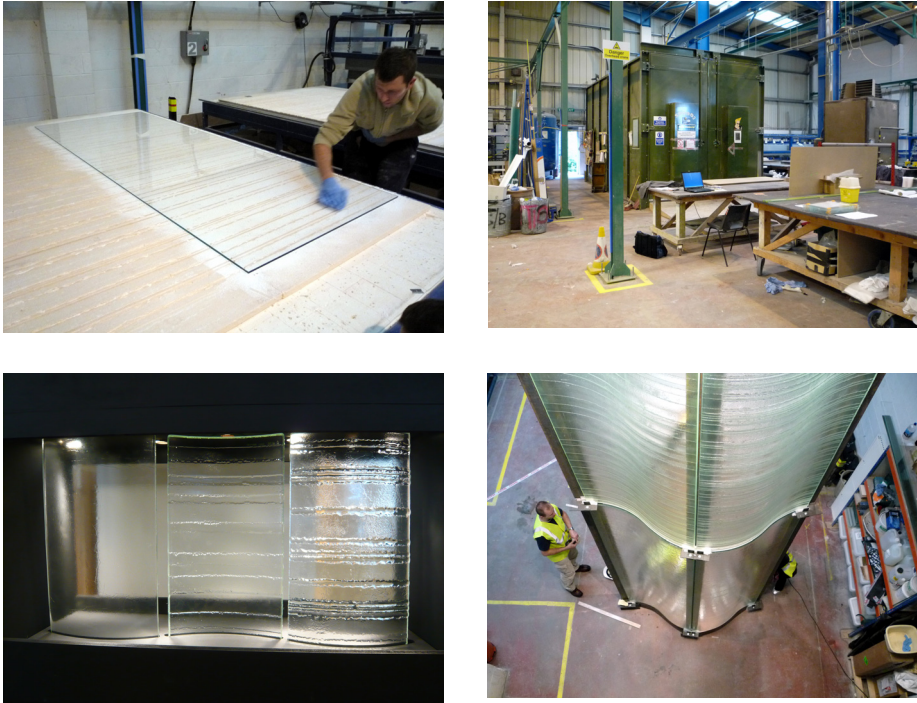
Figure 20a, b, c, d: Sand-bed Glass Texturing, Slumping Oven, Glass Samples, First Lighting Mock-up.
