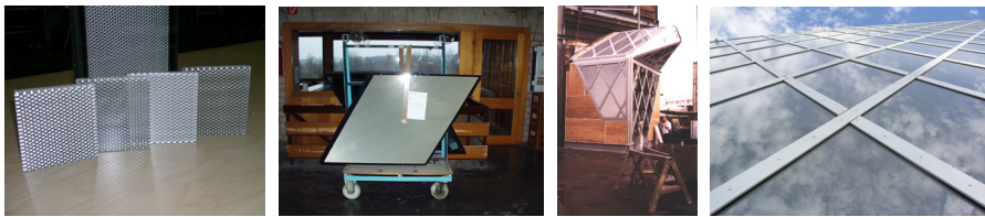
Figure 2a, b, c, d: Mesh-Glass Samples, Production Panel, Performance Mock-Up, Installed Mesh Glass.
