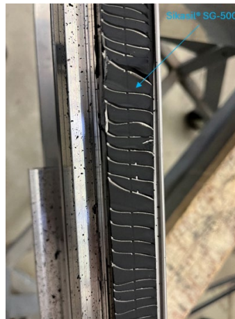
Fig. 21: Sikasil® SG-500 joints after bead adhesion tests showing purely cohesive failure.
