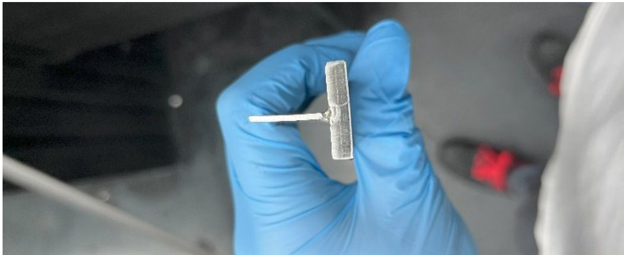
Fig. 2: Example of non-orthogonal welding of the flat steel components of the fitting (Source: Yachtglass).
