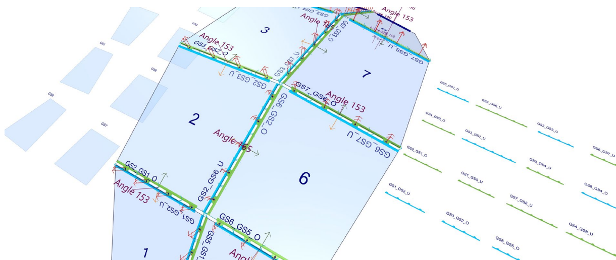
Fig. 20: Close-up of the labelling system, produced by the parametric tool for the assembly of the Glasstec mock-up exhibited in Düsseldorf in 2024 (Source: knippershelbig)
