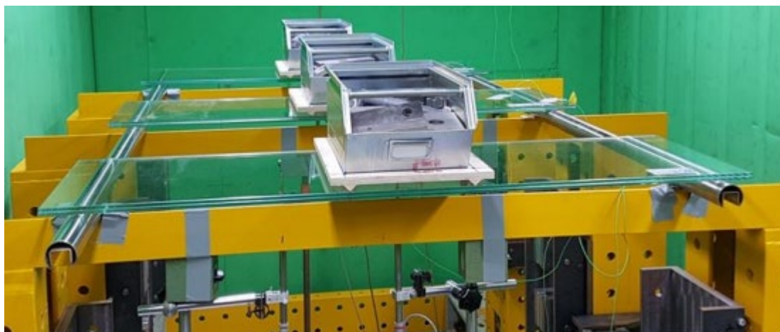
Fig. 3: Four-point bending verification set up in temperature chamber (picture courtesy of Institute of Structural Engineering, University of the German Armed Forces, München, Germany).
