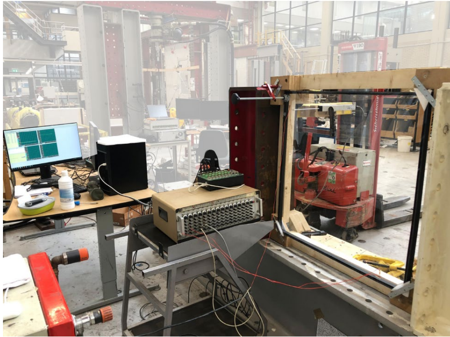
Fig. 4: Setup of the single corner bending tests (own work, 2025)
