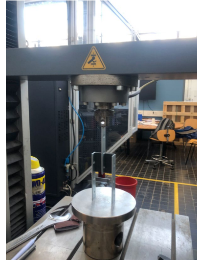
Fig. 3 and 4: result of the tensile test (left) and double-lab shear tests with a piece of spacer between three metal strips. (own work, 2025)
