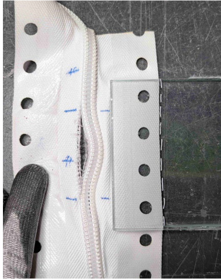
Fig. 2: Tape failure within the clamping zone.
