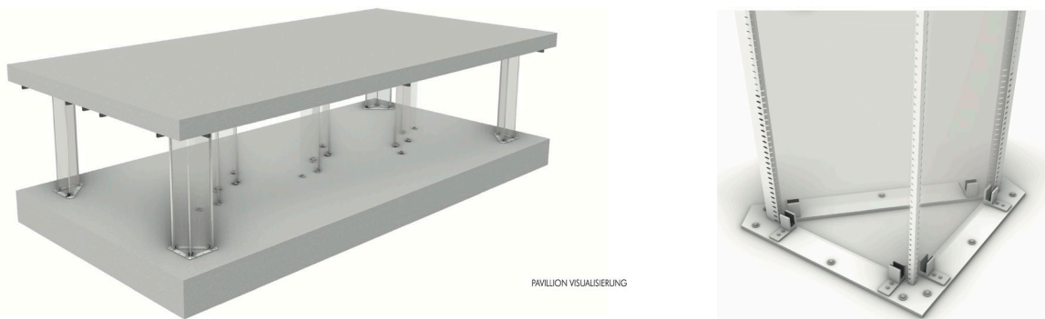
Fig. 4: Glass columns assembled from individual panes using zippers supporting a pavilion roof © van Zütphen, Fernandez, Merkel.
