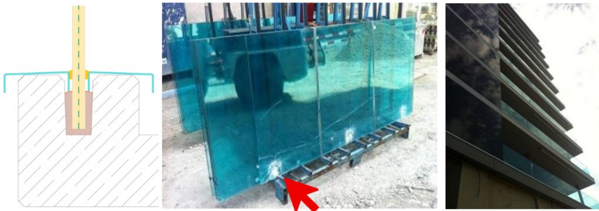
Fig. 3: Nominal line support versus discrete load introduction through local adhesive bonding points.
