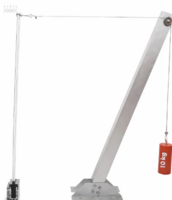
Fig. 6: Simplified test setup with narrower glass and correspondingly reduced weight for evaluating serviceability.
