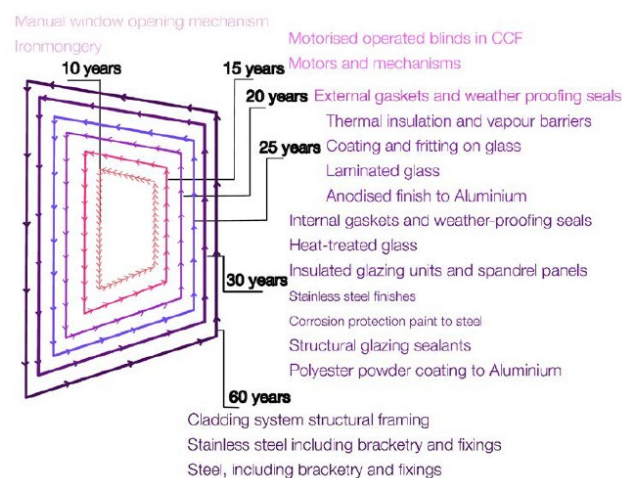
Fig. 1: Lifespan of various components and materials in the façade (Hartwell and Overend, 2019).
