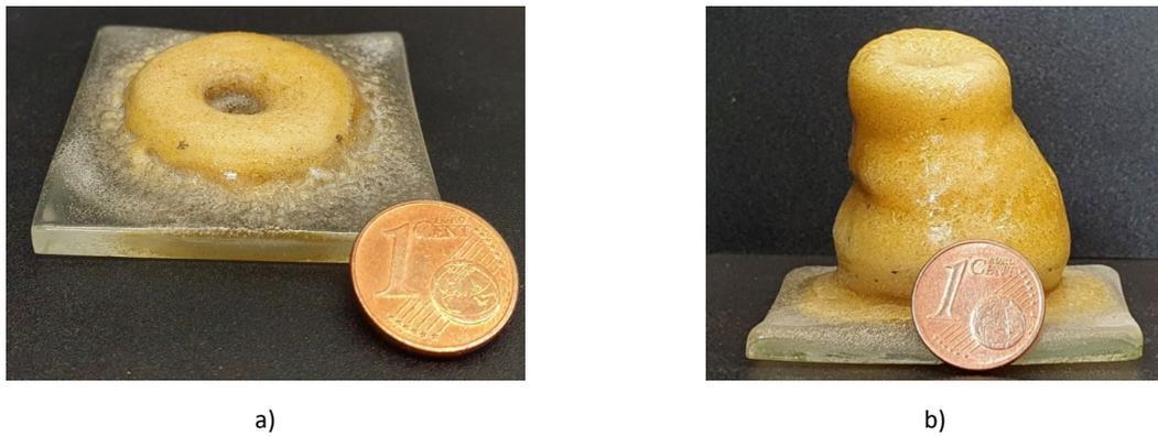
Fig. 5: Samples out of soda-lime silicate glass: a) Sample V5.1 (parameters: 30 mm blue flame cone; distance substrate torch approx. 50 mm); b) Sample V5.3 (parameters: 40 mm blue flame cone; distance substrate torch approx. 50 mm).
