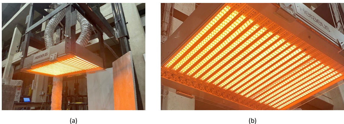
Fig. 2: Radiant panel: (a) Infrared emitters operating at 10% intensity, (b) Close-up of emitters operating at 10% intensity.
