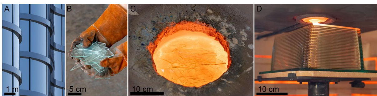
Fig. 5: Process for float glass recycling A) Float glass installed as windows B) Hammer crushed float glass cullet C) Pre-heated glass cullet loaded into the JK kiln D) Recycled float glass extruding onto Optifloat float glass.
