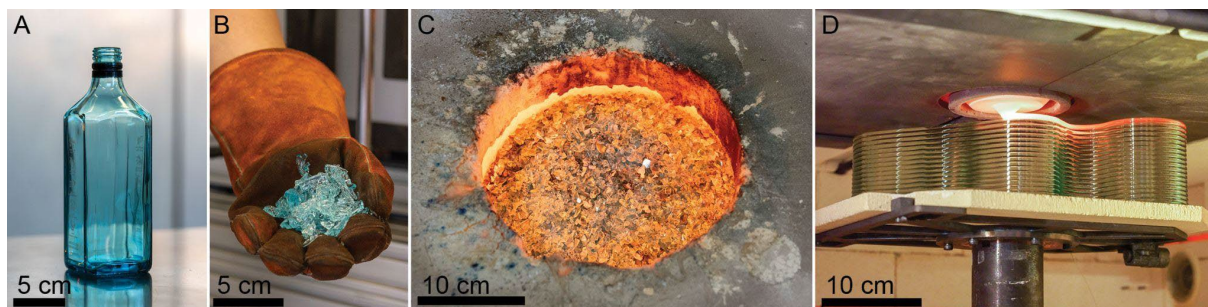
Fig. 4: Process for container glass upcycling A) Sapphire glass container B) Pulverized container glass cullet C) Pre-heated glass cullet charged (loaded) into the JenKen kiln D) Postconsumer container glass extruding from the printer's nozzle.
