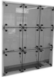
Figure 5 Experimental model of glass. Structural glass panels 1989.
