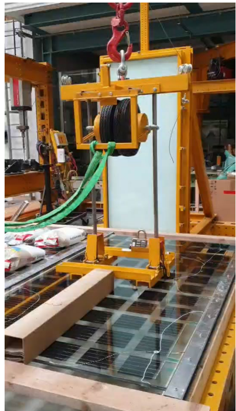
Fig. 6 and Fig. 7: Pendulum impact test (left) and test for accessible glazing.
