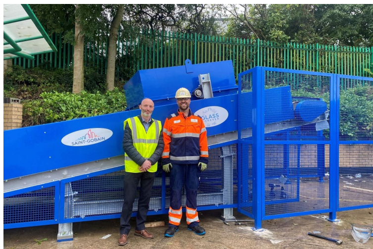
Fig. 1: An example of a high volume crush machine for the reprocessing of end of life domestic glazing from Morley Glass (2022).
