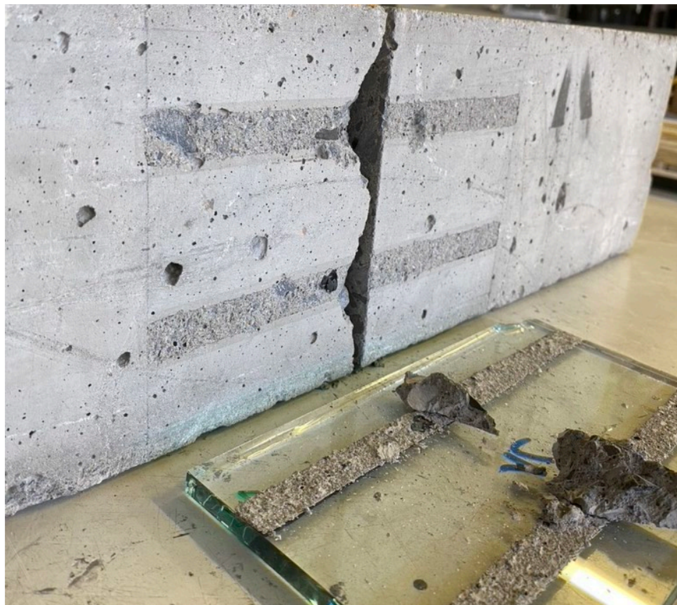
Fig. 10: Failure mode of a specimen with adhesive configuration 3.
