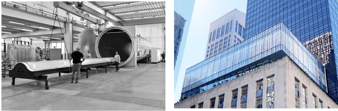
Fig. 9: Glass pane after gravity bending (left) and result of gravity bent glazing at Tiffany & Co. The Landmark flagship store in New York (right) © sedak.
