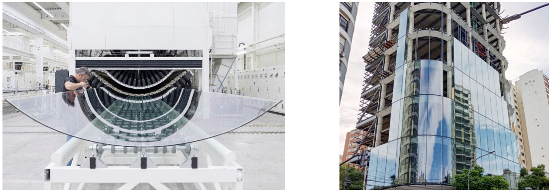
Fig. 7: Glass pane after thermal bending process (left) and result of a thermal bent glazing at a building in Buenos Aires, Argentina (right) © sedak.
