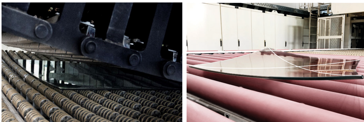
Fig. 1: Image of fully tempered double curved bent glass during (left) and after thermal bending process with indicated curvatures (right) © sedak.
