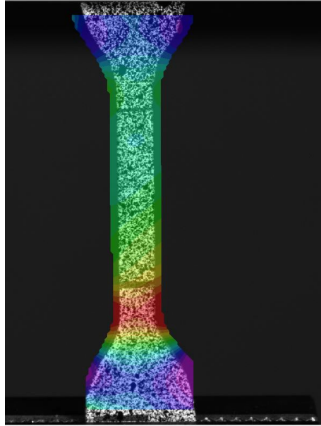
Fig. 5: Longitudinal strain field, computed by DIC software, on the surface of a dumbbell tested in tension at 1 mm/min crosshead speed. Red and purple colours indicate high and low strain regions, respectively.
