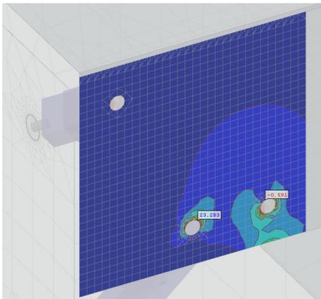
Figure 7: Maximum principal stresses in cross beam at connection.
