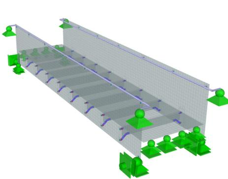
Figure 5: Finite element model of glass bridge.
