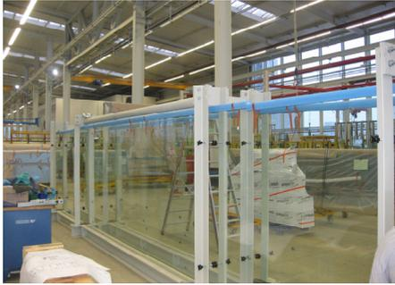
Figure 9: Glass balustrade supported in temporary steel frame.
