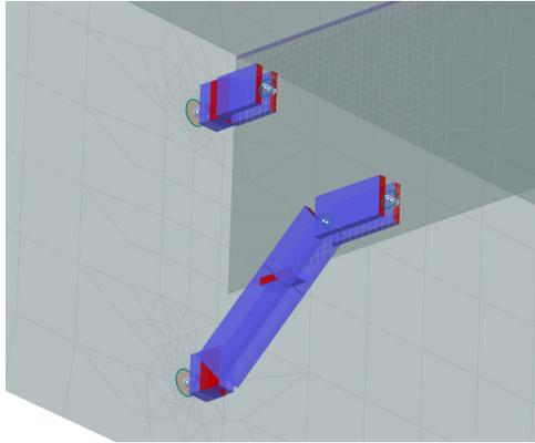
Figure 6: Connection between cross beam and balustrade
