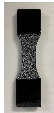
Fig. 5: Dogbone specimen with pattern.
