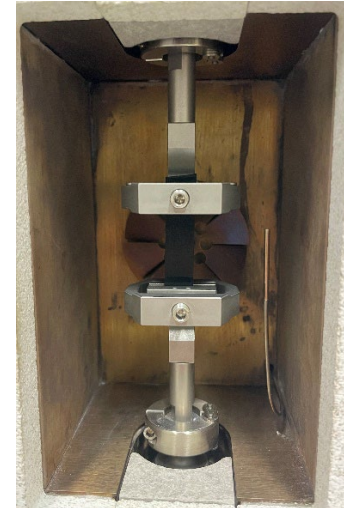
Fig. 2: Installation situation DMTA.
