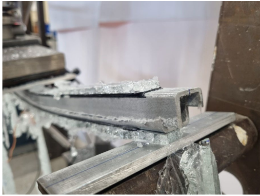
Fig. 7: Horizontal shear failure in GFRP core (specimen A3).
