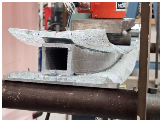
Fig. 9: Horizontal shear failure along the top face of the GFRP core (specimen C1).
