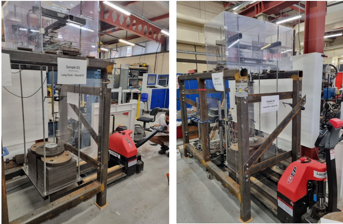
Fig. 4: Long-term loading experimental setup.
