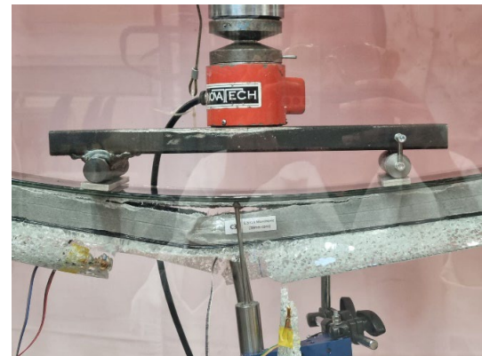
Fig. 10: Second failure in the bottom face sheet (specimen C3).
