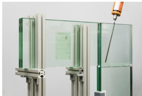
Figure 7: Production studies - application of adhesive to the test specimen with a flat nozzle.
