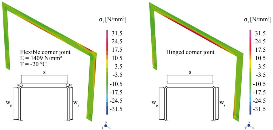
Figure 3: Stress distribution for different states of the structural system.
