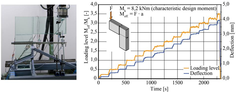
Figure 5: Verification of load bearing capacity: test set-up and results.
