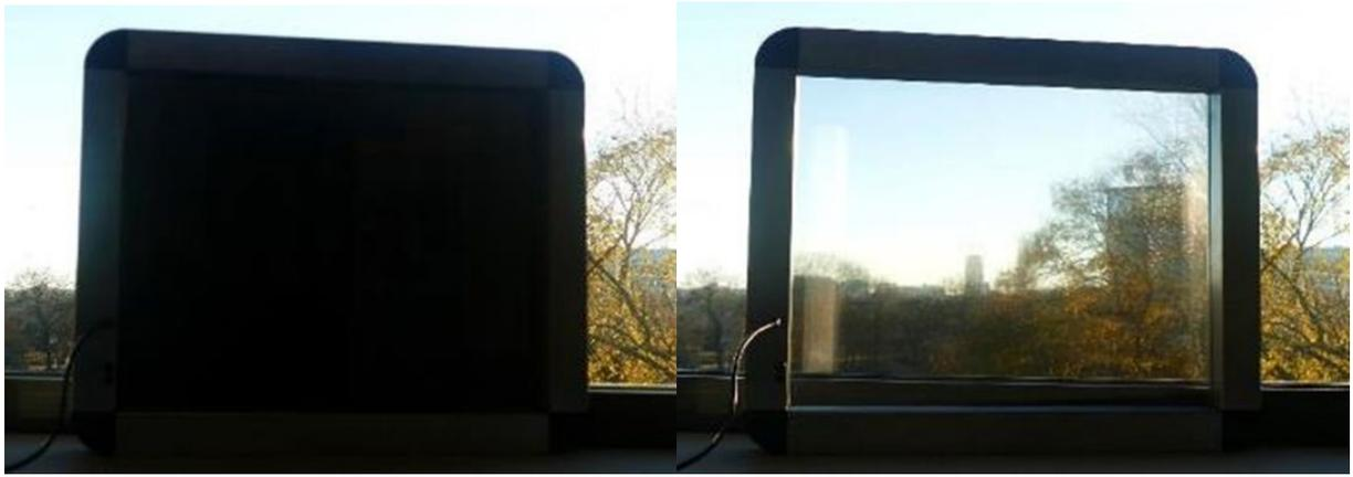
Fig. 2: ELM window in dark state (left) and clear state (right).
