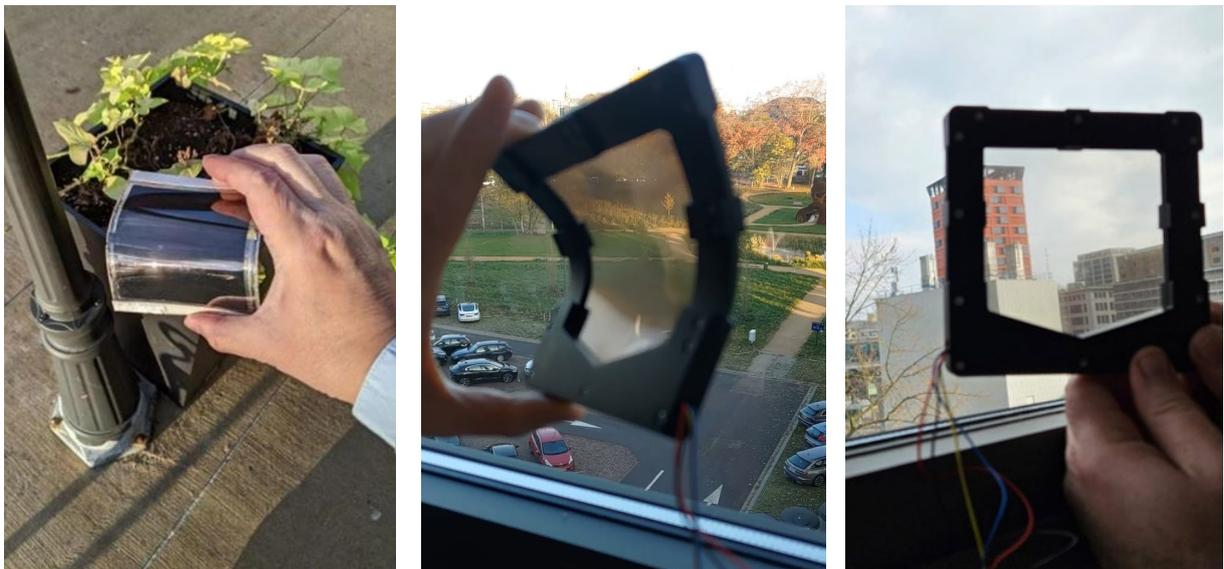
Fig. 3: ELM prototypes based on plastic substrates.
