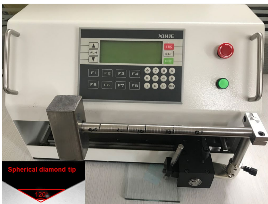
Fig. 1: Configuration of the scratch testing machine.
