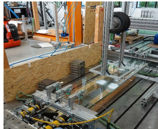
Fig. 9: Testing stand with specimen and vertical twin tire.
