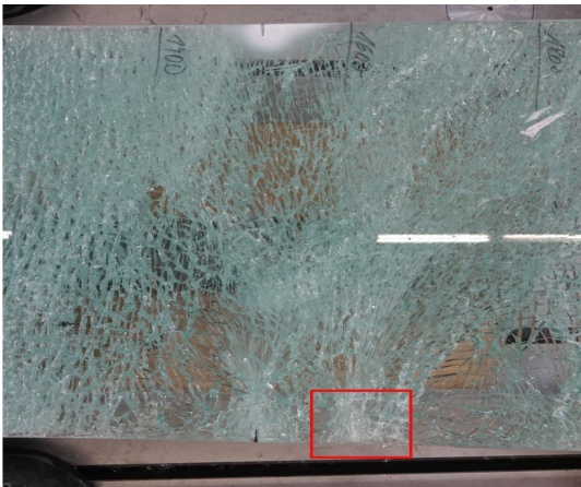
Fig. 21: Fracture pattern and area of origin of the specimen subjected to impact and 75 kN compressive load.
