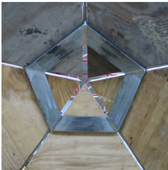
Figure 10: Pentagonal Mock-up of top of the dome in plywood (scale 1:2)
