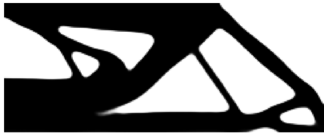
Fig. 4: Optimized half-MBB beam.
